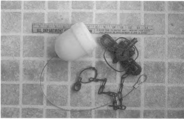
EGG™ trap and No. 1 Victor™ coil spring trap. Length of ruler above trap is 38.1 cm. Photo by George F. Hubert, Jr., Illinois Department of Natural Resources.
