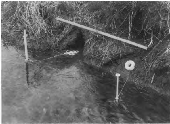
Fig. 2. Paired set used to evaluate raccoon restraining traps in Illinois. For purposes of illustration the traps are set <3 m apart, the anchor stakes for both traps and the EGG™ trap anchor cable are painted white and left exposed, and the No. 1 Victor™ coil spring trap is painted white and exposed above surface of water to show positioning. Length of ruler above traps is 1 m.
