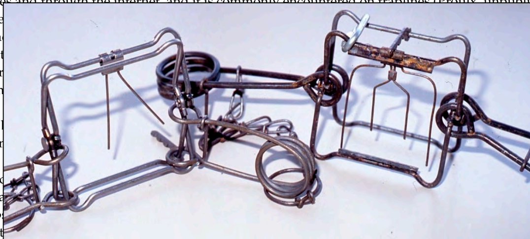
Figure 1. Examples of the Conibear 120 trap with a two-prong trigger (left) and the C120 Magnum trap with a pitchfork trigger (right). Note the larger springs and clamping bars welded to the striking jaws of the C120 Magnum (Photograph: Gilbert Proulx®).
