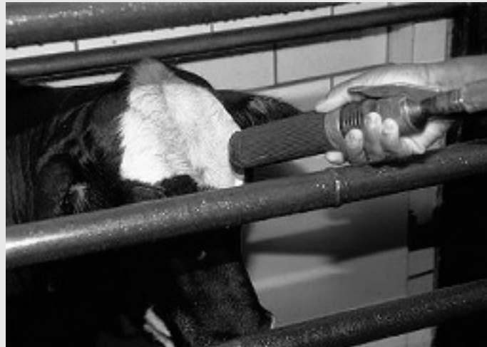
A cow being stunned with a mechanical captive bolt.
