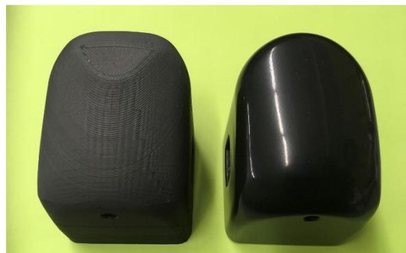
The least time-intensive form of surface finishing is chemical smoothing. The 3D print is exposed to a bath or vapor of a solvent, which causes the surface to flow. The print is removed from the solvent and the solvent is allowed to off-gas, leaving behind the plastic object. As an example, here is a beginner's guide to vapor smoothing from the All3DP educational website <https://all3dp.com/2/abs-smoothing-a-beginners-guide-to-abs-vapor-smoothing/>.
