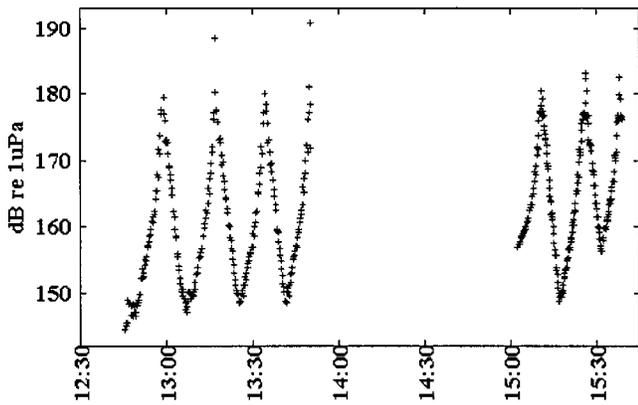
FIG. 1. Received air-gun signal levels with time (lower axis). Units are *mean squared pressure* over the portion of the signal which encompassed 95% of its energy, as measured from the cage bottom. The signal source was moved toward and then away from the cage as described in the text.
